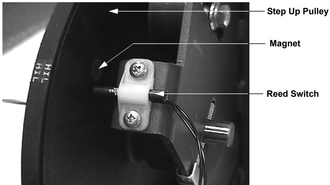
**Diagram 6.4 - Speed Sensor (serial code A998)**
