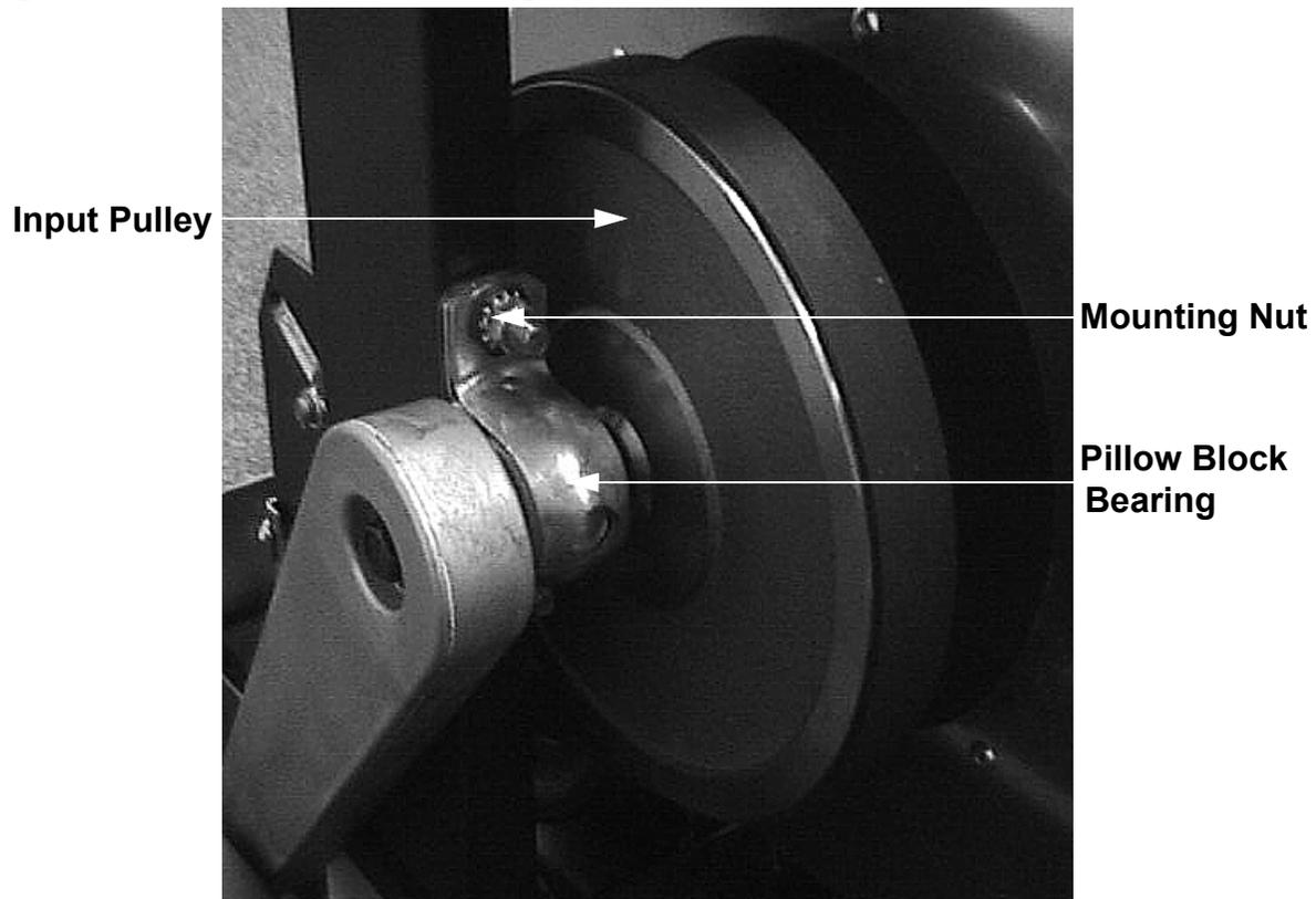
**Diagram 7.10 - Pillow Block Bearings (serial code A998)**
