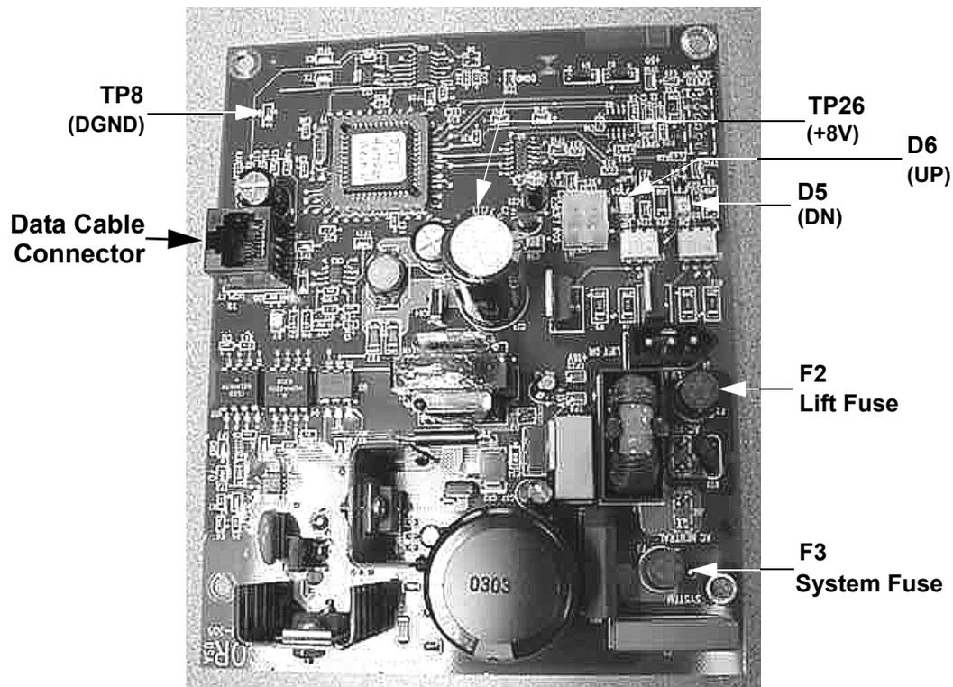
Diagram 6.6 - Lower PCA (Serial code A998)
